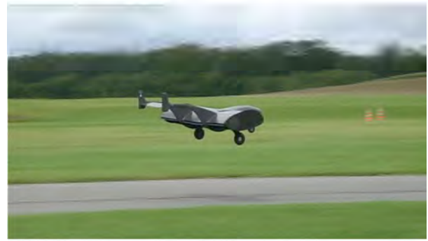
Fig. 3. A cross-flow fan (CFF) unmanned aerial vehicle (UAV) model in flight [5].
