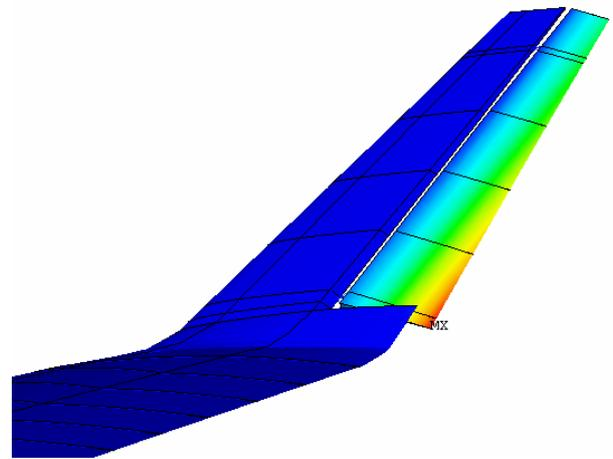
Figure 8: FEM model of winglet with deflected tab
