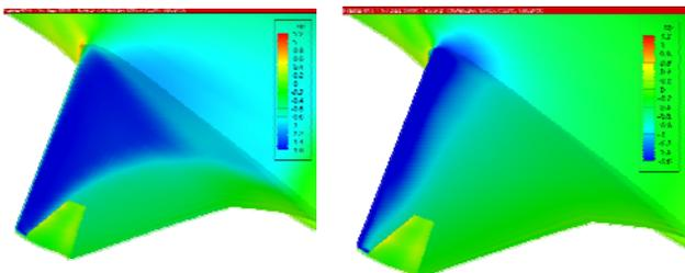
Figure 2: 2,5g load case pressure distribution in a gust in cruise flight conditions and at sea level after pull out of a dive.
