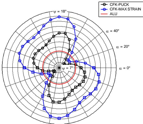
Figure 7: Twist of the winglet in relation to material orientation
