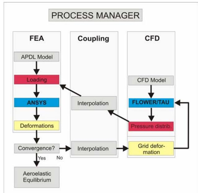
Figure 3: Sequential FEM-CFD coupling
