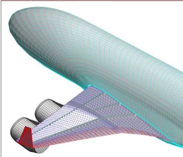
Figure 1: PARA\_MAM FEM wing-winglet model with engine dummies and CFD surface mesh of the fuselage.
