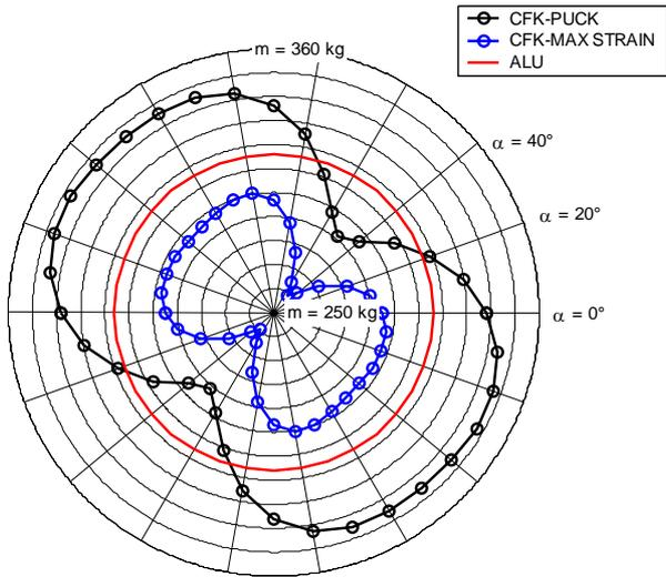
Figure 6: Mass of the winglet in relation to material orientation
