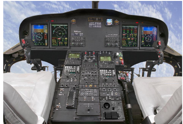
Fig. 7: avionic technology (AB139 cockpit layout)
