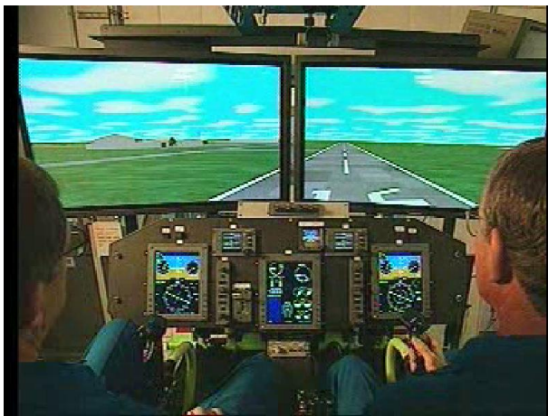
Fig. 26: BA609 Simulation Facility with hardware and pilots in the loop
