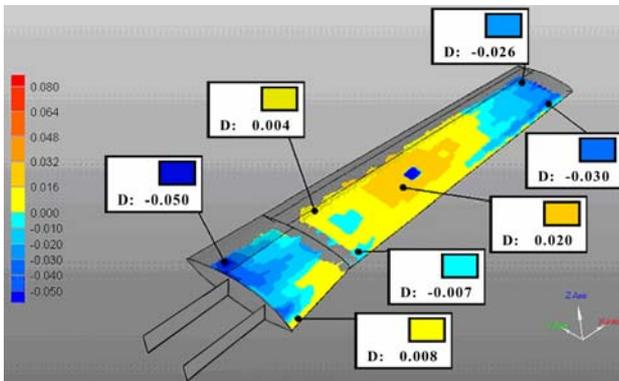
Fig. 10. Upper surface inspection data (inches)
