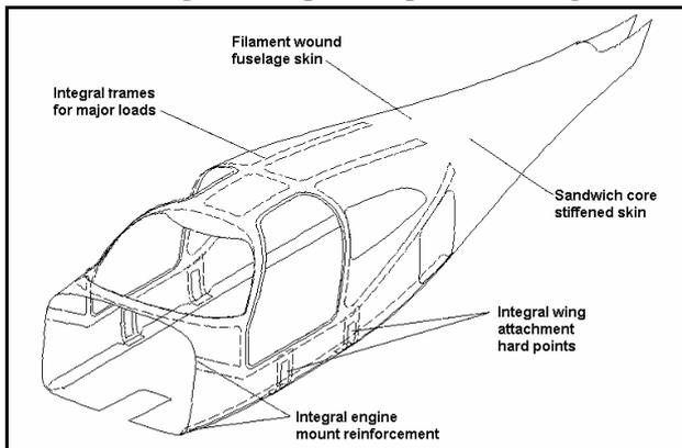
Fig. 3. Initial fuselage concept
