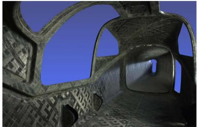
Fig.11. Fuselage interior viewed through firewall opening
