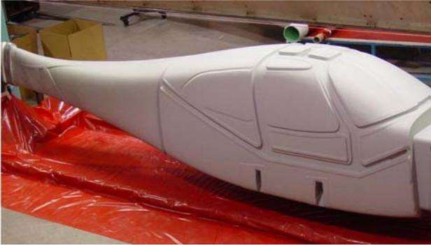
Fig. 7. Fuselage winding mandrel
