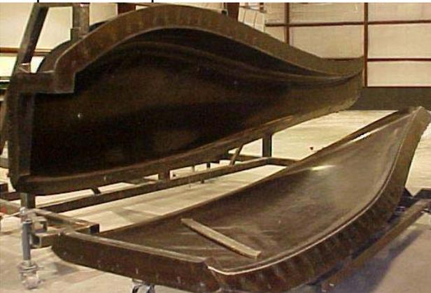
Fig. 8. Right side, bottom and insert of OML Mold
