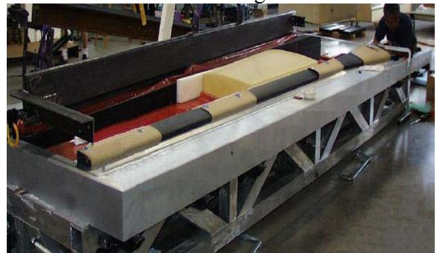
Fig. 6. Wing mold base and some internal tooling
