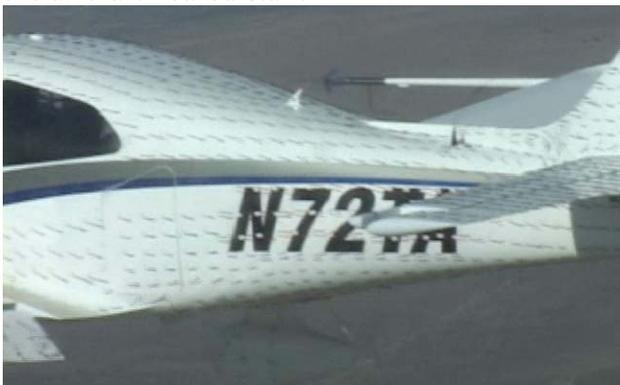
Fig. 13. Air flow over the tufted fuselage surface
