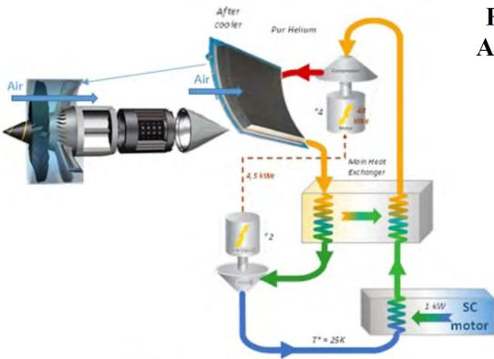
Figure 1: cryocooler cycle with air as hot sink
