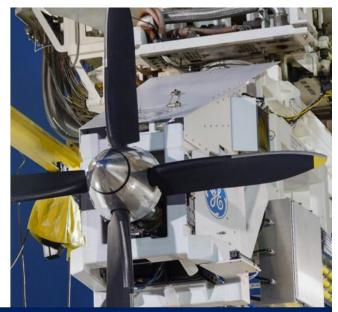
Robust system ground and altitude maturation tests underway to demonstrate flight readiness
