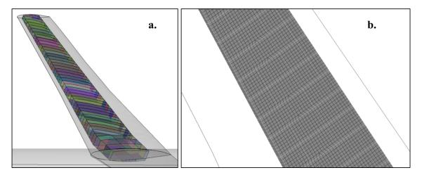
Figure 5 – Internal structure of the wing. a. box layout b. Mesh used for structural analyses of the wing box
