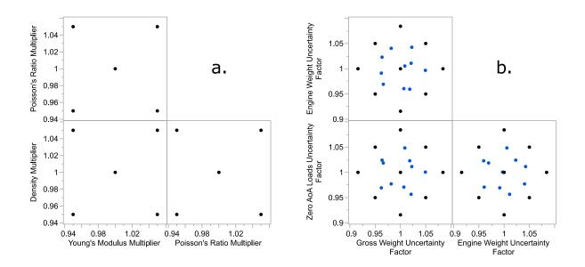
Figure 7 – DoEs used to sample uncertainty factors. A. Central Composite Design b. Full Factorial Design with a center point
