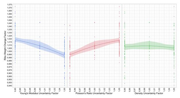
Figure 9 - Impact of wing structure material uncertainty factors on the overall wing weight
