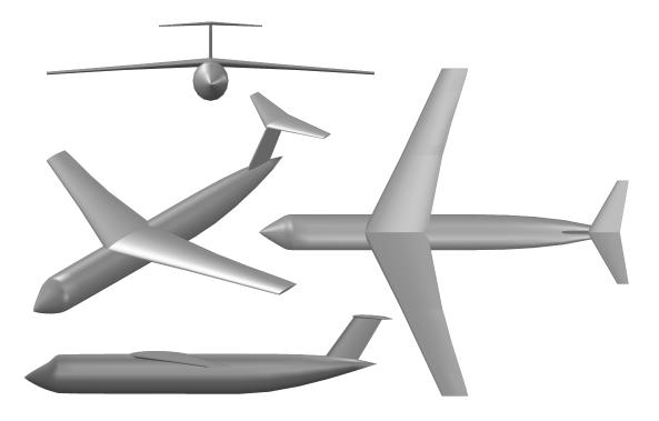
Figure 4 – OpenVSP model of the Lockheed C-5M
