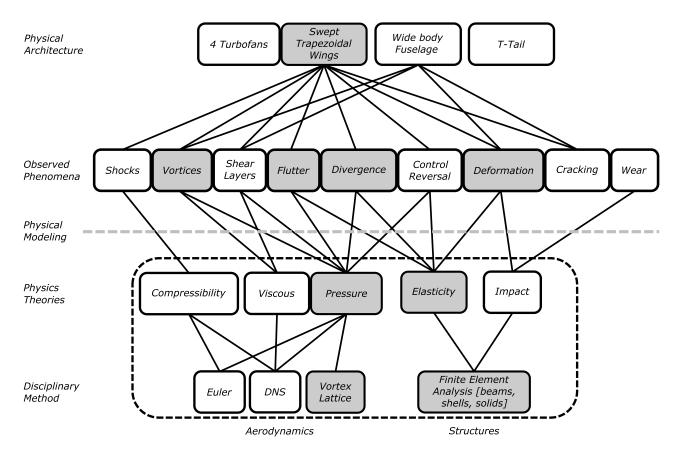
Figure 3 – Modeling architecture from an aerodynamics and structures perspective.
