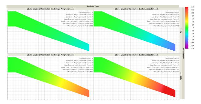
Figure 10 – Wing box deflection due to aerodynamic loads Top row: Load Factor = -1g, Bottom row: Load Factor = +2.25g. Left column: Decoupled Analysis, Right column: Coupled Analysis
