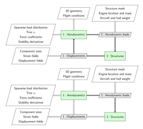
Figure 6 – Two different xDSM approaches for aeroelastic analyses. Decoupled aero-structures (top) and coupled analyses (bottom)
