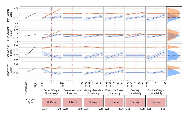
Figure 11 – Prediction profiler for parameter uncertainties (decoupled analysis in orange, aeroelastic analysis in blue)
