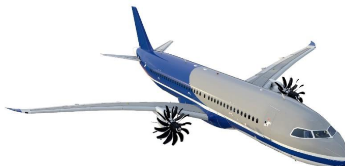
Figure 12 : Example of a LW installation of the Open fan (illustration purpose)
