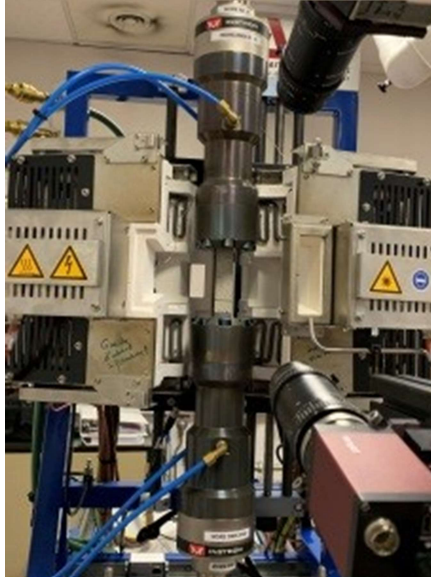
Fig. 5: High temperature set-up for testing composites
