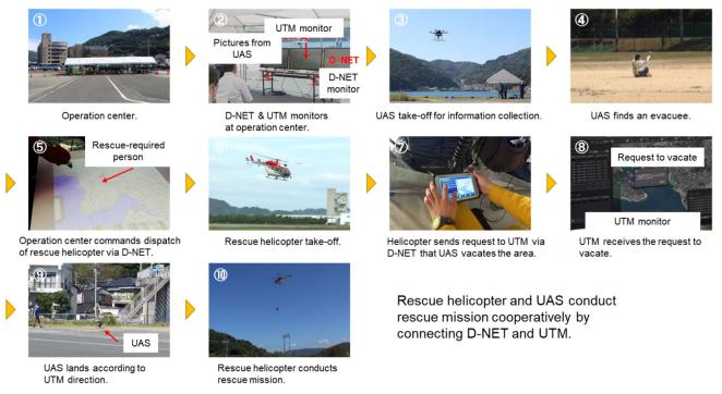
Fig. 9 Cooperative rescue mission of manned helicopter and UAS by connecting D-NET and UTM.
