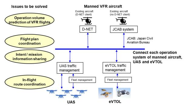
Fig. 6 Concept of integrated operation of manned aircraft, eVTOL and UAS.
