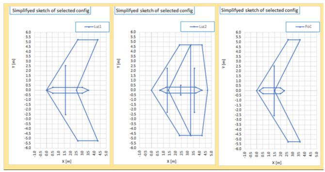
Figure 14 - The simplified geometries defined for the 2 configurations and the PoC, obtained from the Conceptual Design Studies.
