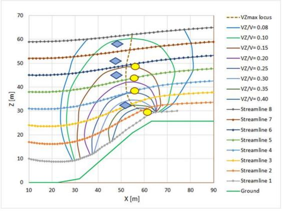
Figure 12 - Positioning of 4 characteristic HG in the Wind field of the previous figure. The Rhombi correspond to wind of 25 km/h and the ellipses correspond to 18 km/h.
