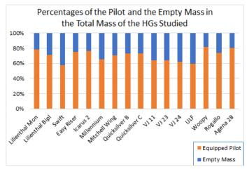
Figure 9 - Percentages of the Pilot and the Empty Mass in the Total Mass of the Hang Gliders
