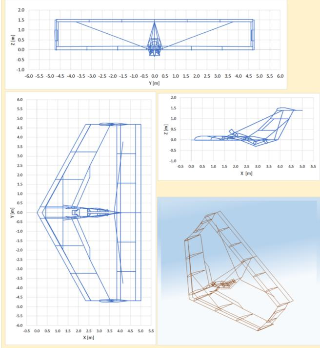
Figure 16 - Views of the 2<sup>nd</sup> configuration, "Conf 2" proposed after preliminary design.
