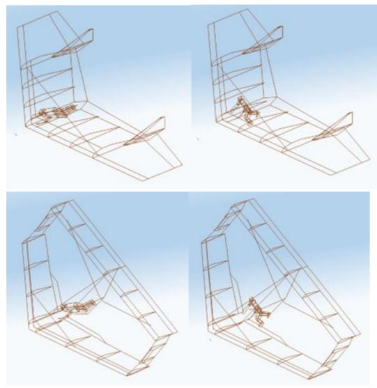
Figure 18 - Positioning of the pilot during ground run (left) and flight, for the 2 configurations.
