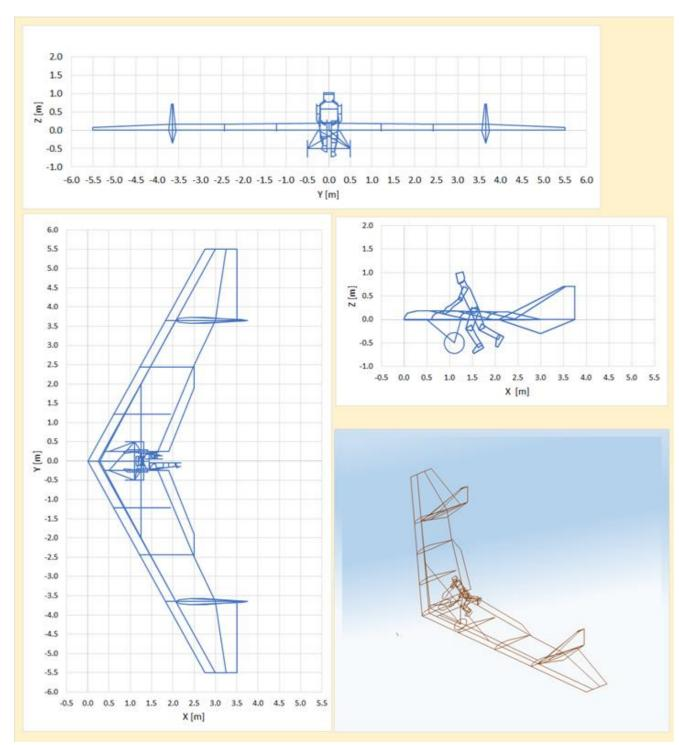
Figure 17 - Views of the PoC proposed after preliminary design.
