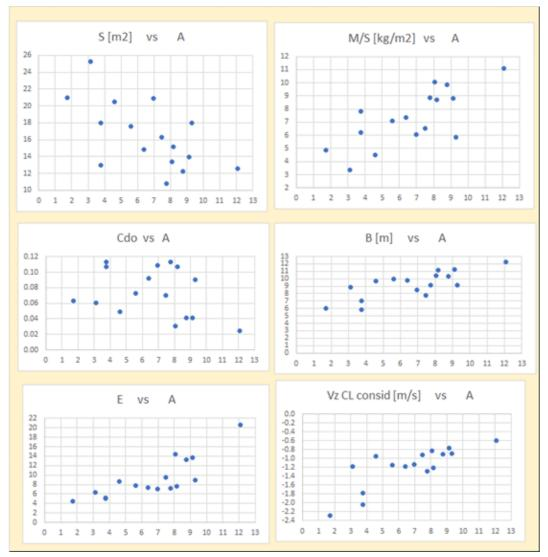
Figure 6 - Characteristics obtained from the HG studied, in function of the aspect ratio.
