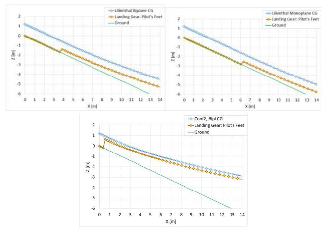
Figure 20 - One Detail of the take-off for 3 gliders: The take-off run.
