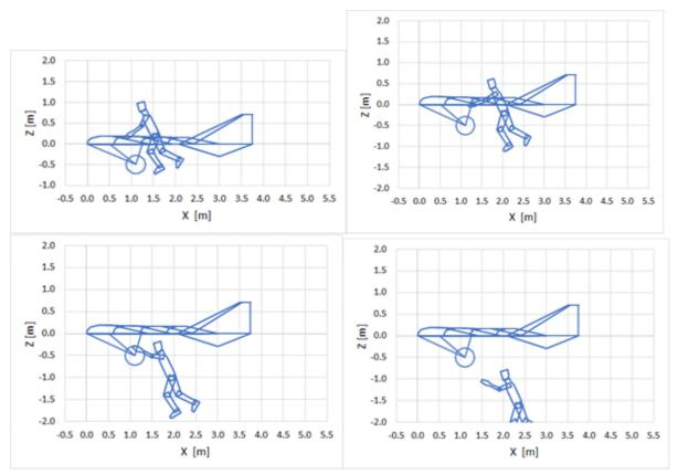
Figure 23 - Sequence of relative positionings between launcher and the PoC during PoC take-off.
