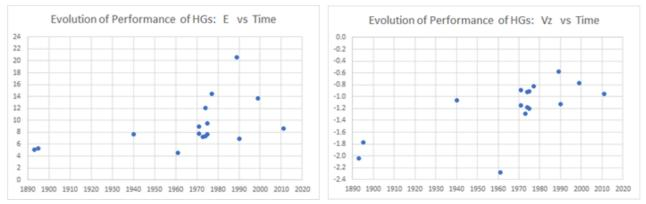
Figure 8 - Historical Evolution of Glide Ratio *E* and Sinking Ratio *VZ* in Hang Gliders
