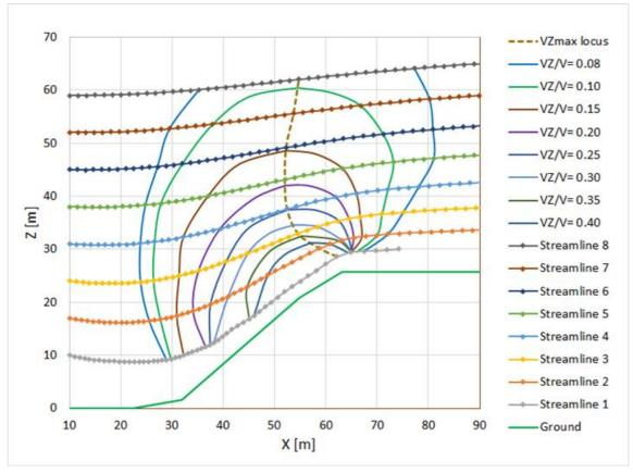
Figure 11 - Aerology Model: Wind, facing a ramp-shaped ground, Streamlines and distribution of Wind Vertical Speed Ratio *VZ/V*.
