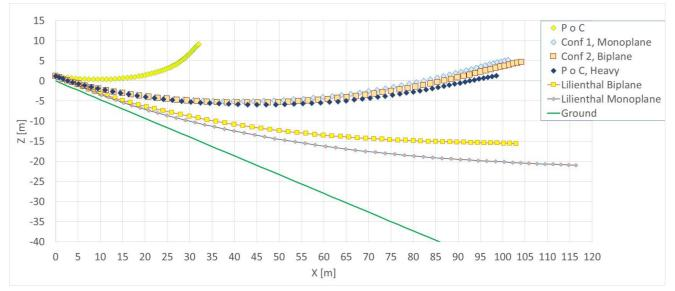
Figure 19 - Simulated Take-off of 5 gliders from a ramp subjected to constant front wind of 10 km/h.
