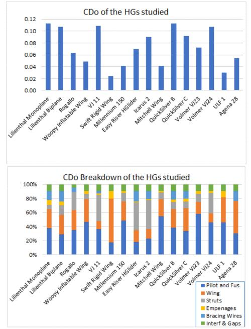
Figure 4 - Comparison of *CDo* of the aircraft studied and the Breakdown of the *CDo*
