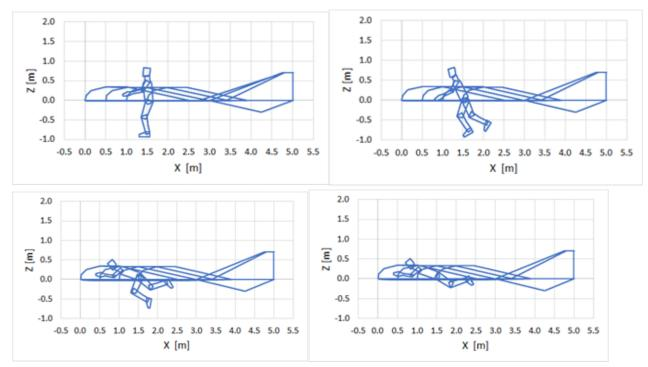
Figure 21 - Configuration 1, Sequence of positionings of the pilot from ground handling, ground take-off run, transition, and flight, from upper left to lower right.
