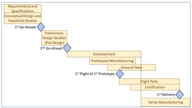
Figure 2 - Aircraft Generic Development and Production Plan
