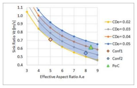
Figure 13 - Sinking Ratio vs Aspect Ratio for several CDo's. also presenting the design space
