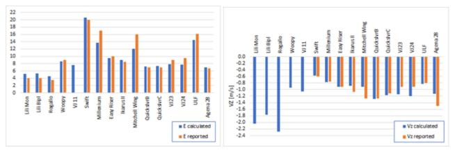
Figure 5 - Calculated and Reported values of Glide Ratio E, and Sinking Ratio VZ.
