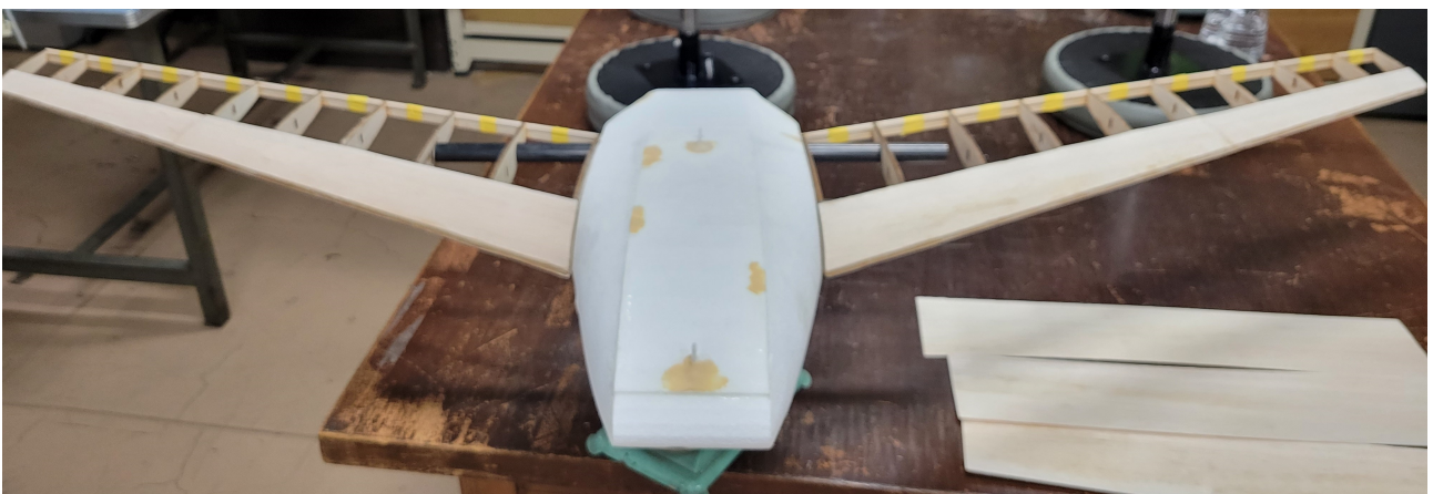
Figure 11 – Experimental UAV in the process of manufacturing
