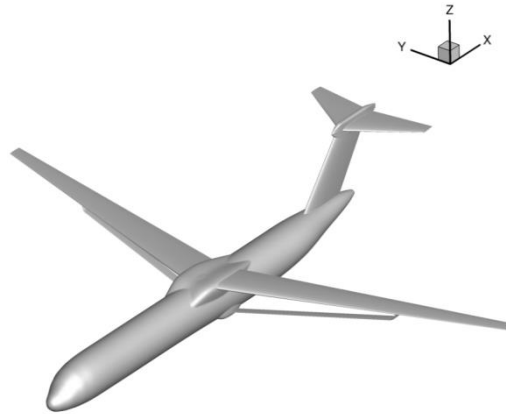
Figure 3. Strut-Braced Wing - Geometry modelling of the reference SBW AR = 16 configuration.
