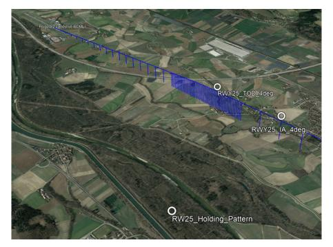
Figure 6 - Planed approach trajectory for EDML RWY 25
