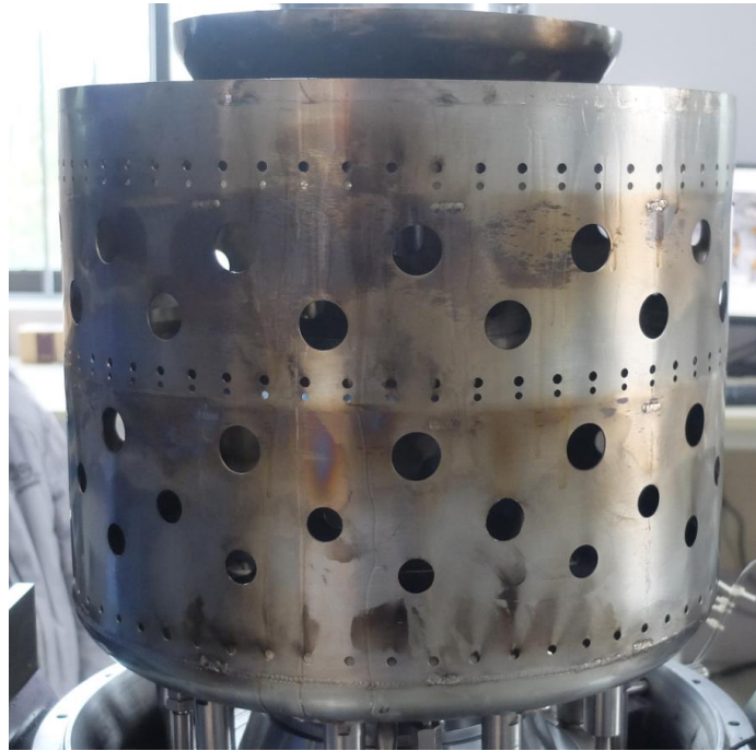
Figure 9 – Combustor manufacture and tests results
