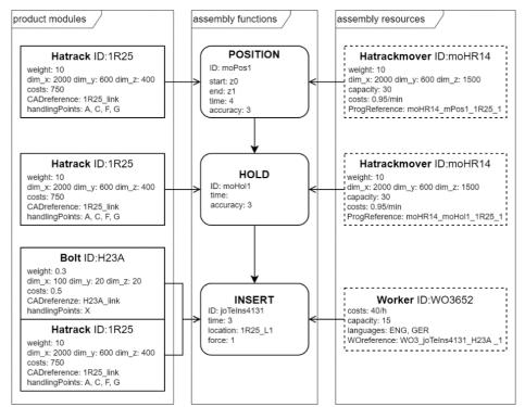
Figure 6 - Excerpt of an example assembly sequence
