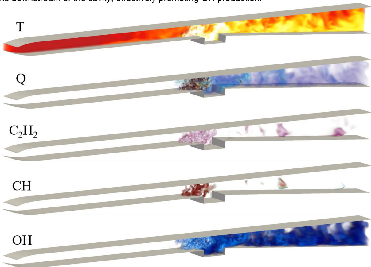
Figure 12 - Volumetric rendered temperature, heat release, C_2H_2 , CH and OH along the centerline of the x-axis, at an instant where the flame is jet-wake stabilized.
