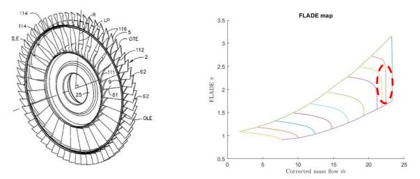
*Figure 2: Left: FLADE geometry showing the outer and inner sections of the geometry [15]. Right: A FLADE map obtained by scaling.*
