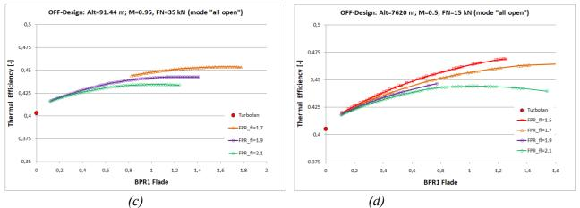
*Figure 4: BPR1 Effect on the ACE thermal efficiency for "all open" mode at the off-design conditions: (a) Case No 01; (b) Case No 02; (c) Case No 03; (d) Case No 04.*
