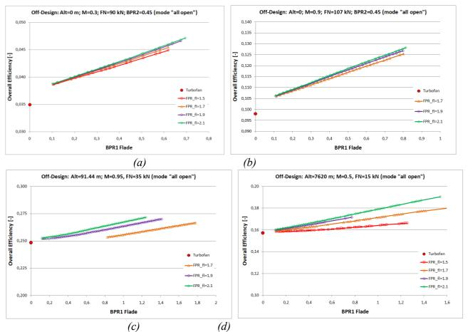
*Figure 6: BPR1 Effect on the ACE overall efficiency*  $(\eta T * \eta p)$  *for "all open" mode at the OFF-Design conditions: (a) Case No 01; (b) Case No 02; (c) Case No 03; (d) Case No 04.*
