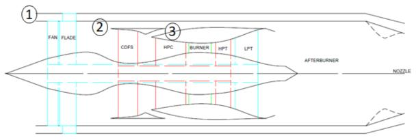
Figure 1: Schematic sketch for ACE engine architecture
