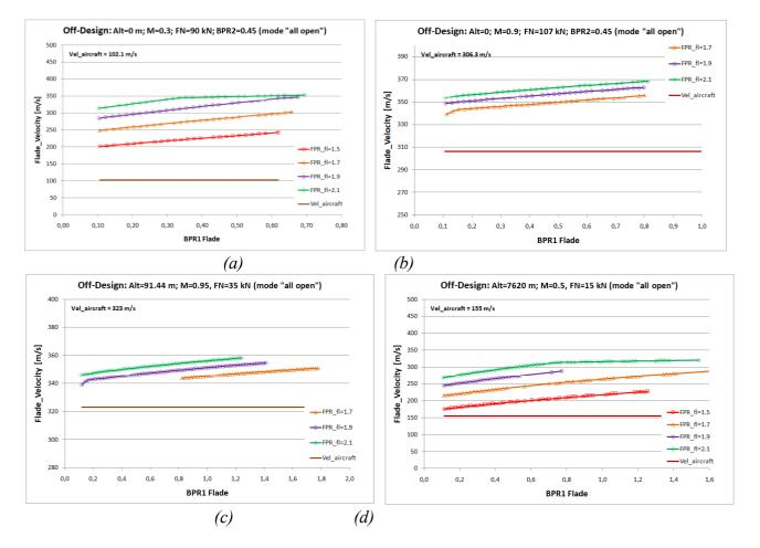
*Figure 8: BPR1 Effect on the ACE FLADE velocity for "all open" mode at the off-design conditions:* (*a*) *Case No 01; (b*) *Case No 02; (c*) *Case No 03; (d*) *Case No 04.*
