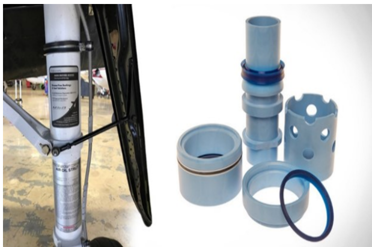
Figure 1 - Polymer landing gear bushings [20].
