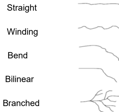
Figure 12 - Schematic of typical crack features, adopted from [30].
