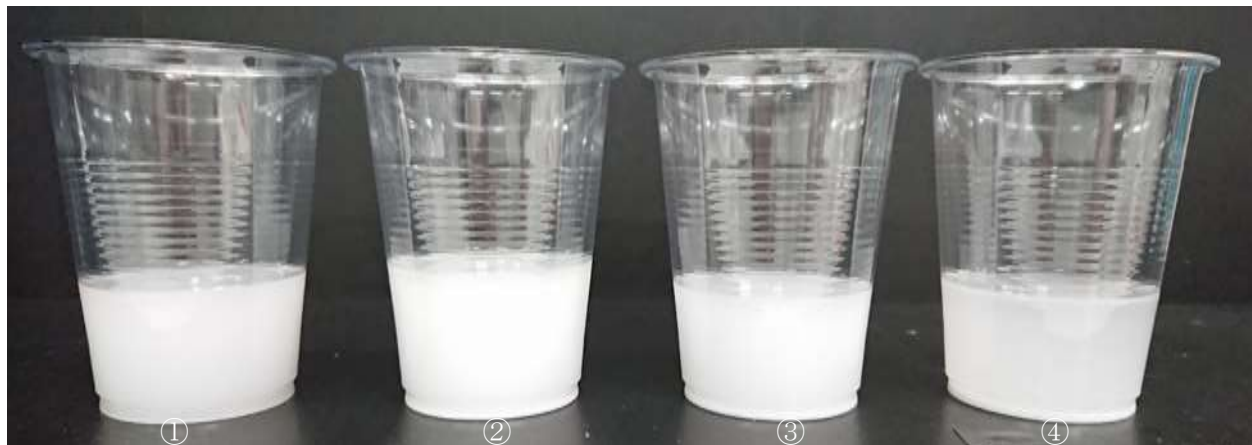
Fig. 8 The state of the emulsified fuel after 1 hour stirring
