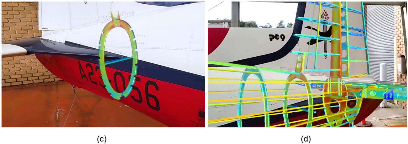
Figure 4 – (a) Decommissioned PC-9/A testbed aircraft at RMIT University; (b) Researcher performing AR-NDE inspection of PC-9/A aft fuselage and empennage using HMD; (c) HMD AR view of Frame 9 Fatigue Damage Index Map positioned in-situ on real aircraft; (d) HMD AR view of full internal empennage structure Fatigue Damage Index Map overlaid on aircraft.
