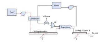
Figure.1. Rankine cycle TMS utilizing fuel as the working fluid [4]
