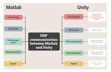
Figure 4 – Communication diagram.
