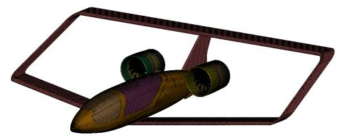
Figure 3 Meshed aircraft model
