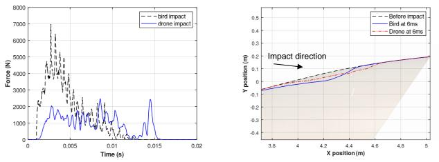
Figure 13 Force vs time comparison between bird and drone impacts on the canopy and, deflection plot
