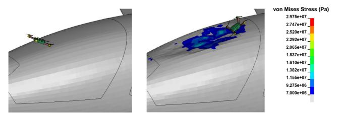
Figure 8 Drone impact on the canopy
