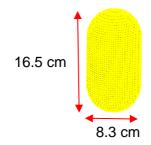
Figure 5 Cylindrical SPH bird impact model.
