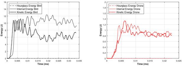
Figure 18 Energy-time history for bird and drone impacts on the fuselage
