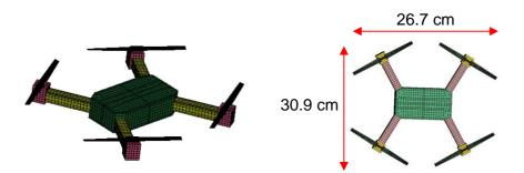
Figure 6 Drone impact model with an equivalent mass to the surrogate bird
