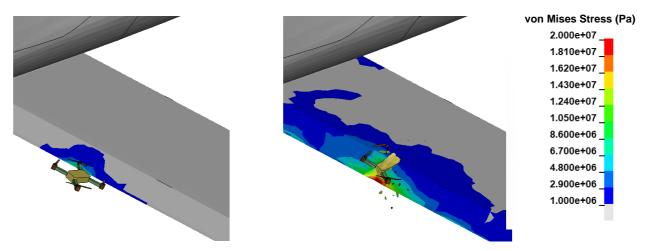
Figure 11 Drone impact on the wing
