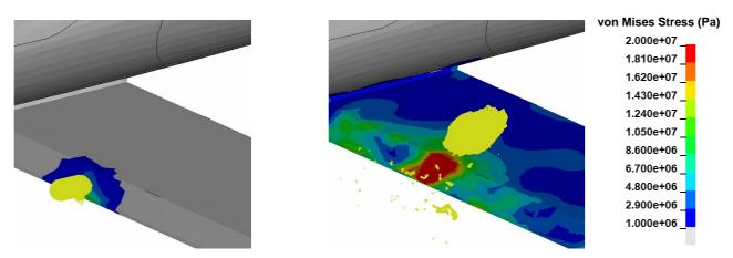
Figure 12 Bird impact on the wing
