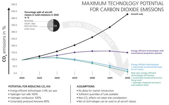
Figure 3. Aircraft emissions can be decoupled from the growth of air traffic through a combination of energy-efficient technologies and sustainably produced kerosene and hydrogen.
