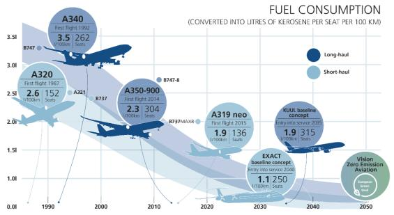
Figure 1. Air transport emissions per passenger per 100 kilometres have fallen continuously over recent decades. New aircraft concepts, such as those being developed as part of DLR's EXACT and KUUL projects, promise further potential emission cuts.
