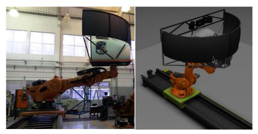
Figure 3. SIVOR flight simulator (cabin with embedded visual system on a robot arm).
