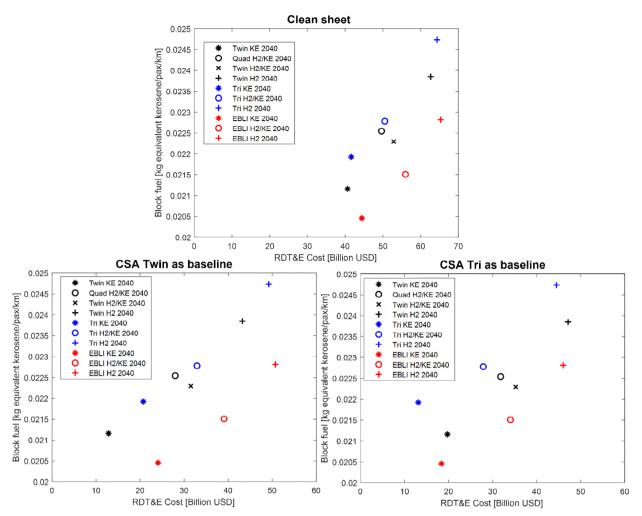
Figure 7: EIS 2040 concepts – performance (in terms of block fuel consumed in kg equivalent kerosene) vs cost for different evolution strategies (Clean sheet, CSA Twin as baseline, and CSA Tri as baseline).
