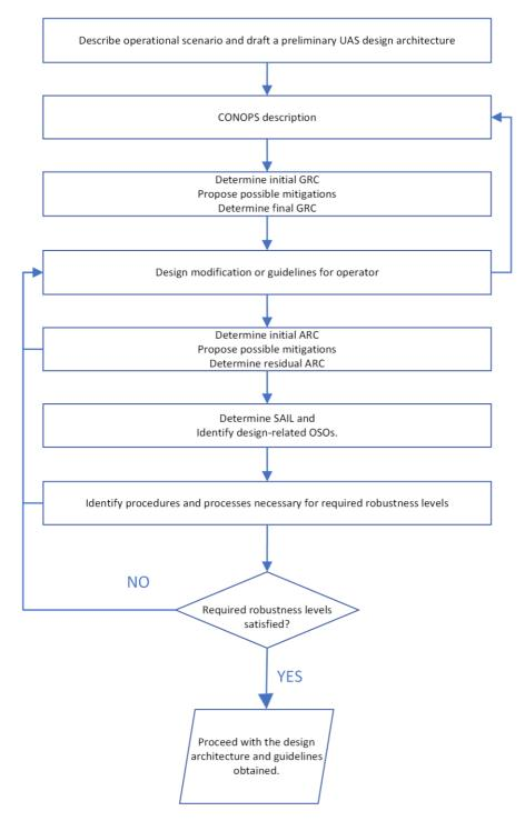
Figure 1 Proposed enhanced UAS design methodology
