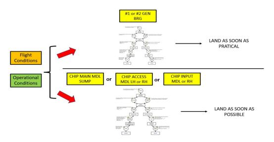
Figure 15. Schematic decision ladder for gen BRG light and one of the CHIP ACCESS MDL LH/CHIP INPUT MDL LH /CHIP MAIN MDL SUMP lights emergencies.
