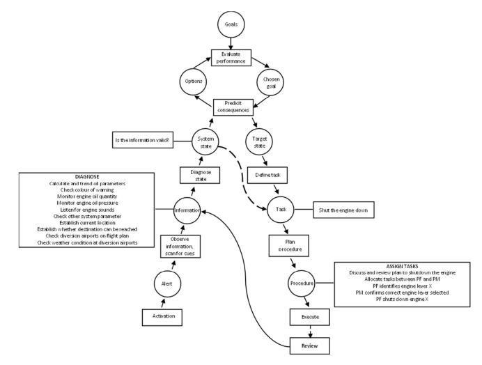
Figure 8. Shortcuts on the decision ladder for an emergency oil leak in an aircraft engine. Adapted from [5].
