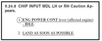
Figure 3. Description of actions related to the chips in the input module emergency [2].
