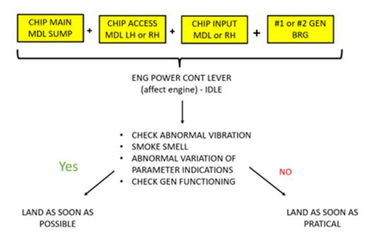
Figure 16. Emergency proposal to be evaluated for lights GEN BRG with CHIP ACCESS MDL LH, CHIP INPUT MDL LH and CHIP MAIN MDL SUMP.
