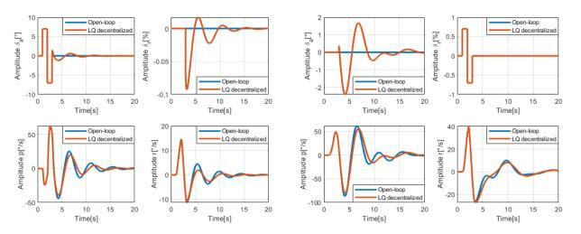
Figure 7 – Response to the 7-degree aileron doublet input (Decentralized).
