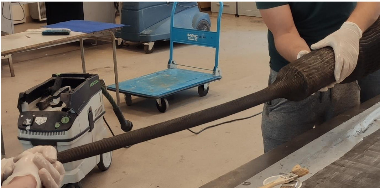
Figure 13 – Outer layer application process.
