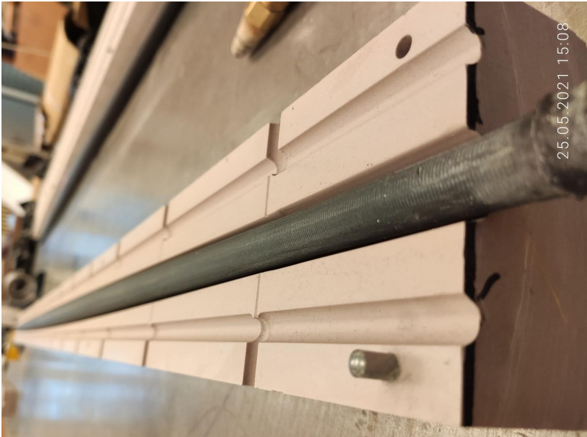
Figure 11 – The mould and the inner core.
