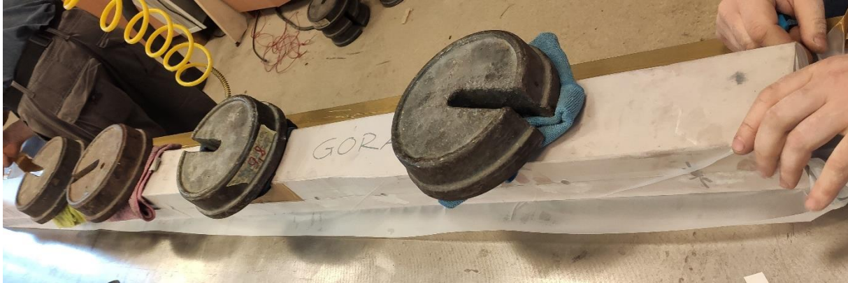
Figure 14 – Closed and sealed mould.
