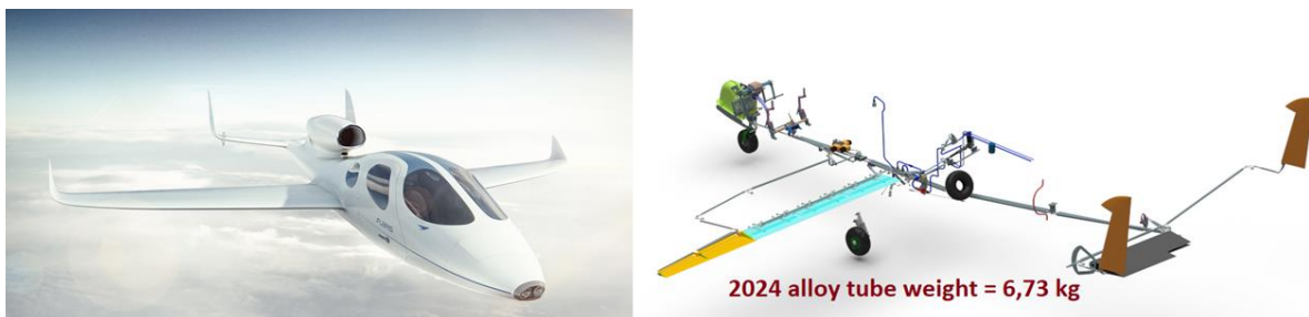
Figure 2 – Small aircraft control system mechanism - four-seater.
