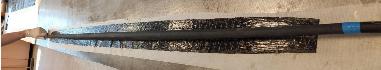
Figure 12 – Unidirectional layer prepared for layering on the core.
