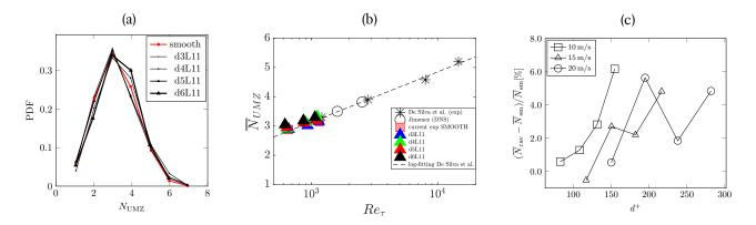
Figure 8 – UMZ for the perforated case, a) PDF of the number of UMZs detected at 20 m/s, b) average number of uniform momentum zones detected for the three flow conditions c) percentage variation of the  $\overline{N}_{\text{UMZ}}$  with respect to the smooth baseline case.
