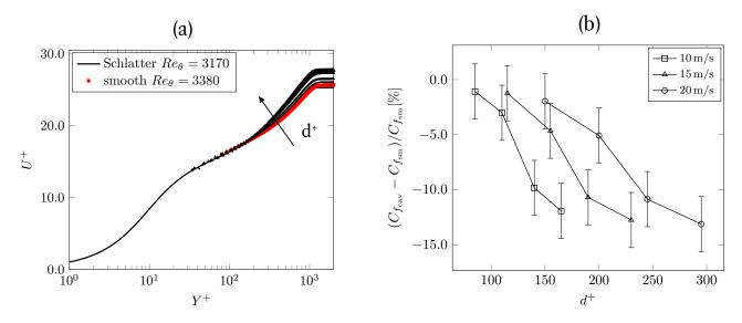
Figure 2 – a) Mean streamwise velocity in wall units at 20 m/s, actual friction velocity is used, size of markers represents the increase in  $d^+$  indicated by the arrow, b) skin friction coefficient percentage variation.
