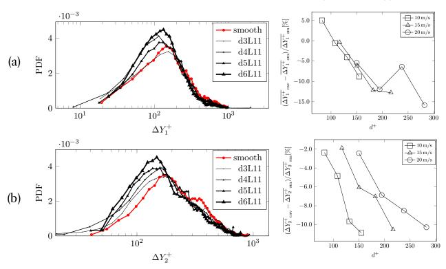
Figure 9 – PDF of vertical extension of the UMZs at  $20 \text{ m/(s (left), and percentage variation with respect to the smooth baseline case (right), a) first zone detected, b) second zone detected.$
