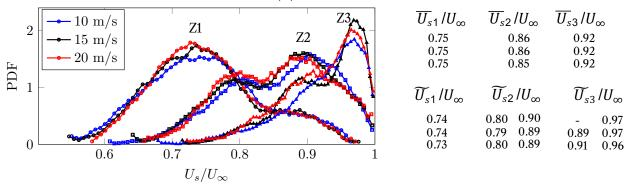
Figure 7 – PDF of the a) modal velocities, b) separation velocities of the UMZs, smooth baseline case.
