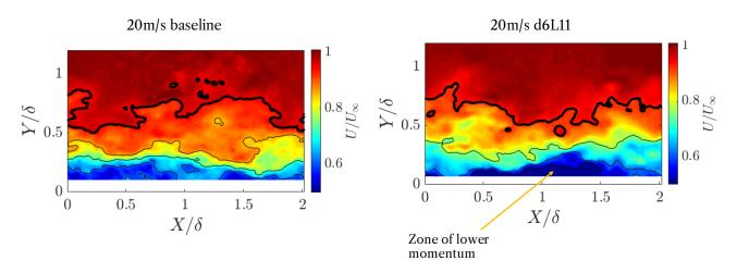
Figure 10 – Randomly chosen PIV snapshots, UMZ detection, a) smooth surface at 20 m/s, b) d6L11 at 20 m/s, flow from left to right.
