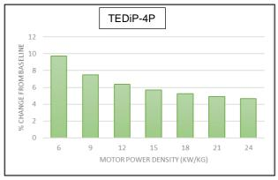
Figure 10. Change in MTOW (%) over baseline for TEDiP-4P with increasing motor power density
