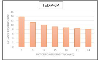
Figure 13. Change in MTOW (%) over baseline for TEDiP-6P with increasing motor power density
