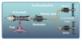
Figure 2. Turbo-electric architecture schematic [2]
