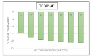
Figure 11. Change in TOFL (%) over baseline for TEDiP-4P with increasing motor power density
