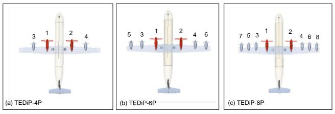
Figure 9. Three variants of ATR 72-500 with TEDiP systems
