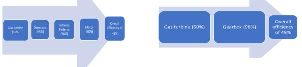
Figure 3(a). Schematic of turbo-electric system efficiency
