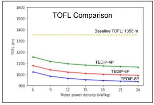
Figure 20. Change in TOFL for TEDiP variants with increasing motor power density
