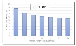
Figure 16. Change in MTOW (%) over baseline for TEDiP-8P with increasing motor power density
