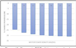
Figure 17. Change in TOFL (%) over baseline for TEDiP-8P with increasing motor power density
