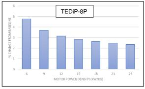
Figure 18. Change in trip fuel (%) over baseline for TEDiP-8P with increasing motor power density
