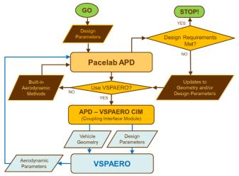
Figure 6. VSPAERO-Pacelab APD Coupling
