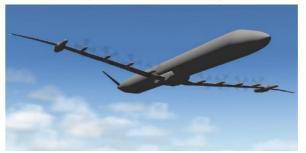
Figure 1. Rolls-Royce Distributed Open Rotor Aircraft concept for regional aircraft. © 2016 Rolls-Royce, plc.
