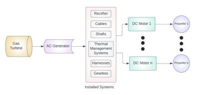
Figure 8. TEDiP system architecture
