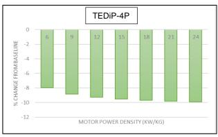
Figure 12. Change in trip fuel (%) over baseline for TEDiP-4P with increasing motor power density
