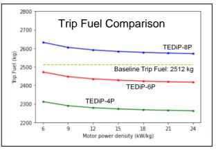
Figure 21. Change in trip fuel for TEDiP variants with increasing motor power density
