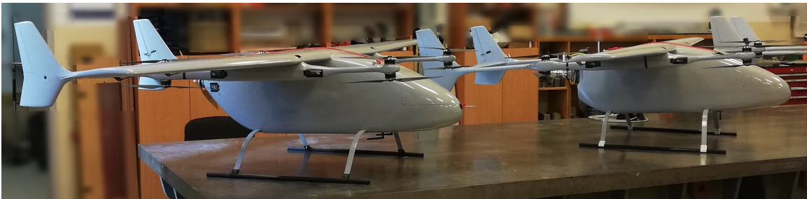
Figure 7 – Two PW Chimera: full electric (left), mixed propulsion (right)
