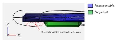
Figure 12 – Possible zone for an additional fuel tank in the front part of the central body.
