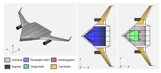
Figure 10 – BWB1 optimized configuration 3D view.
