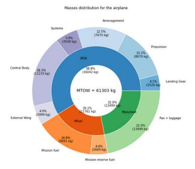
Figure 16 – SMILE configuration mass breakdown.
