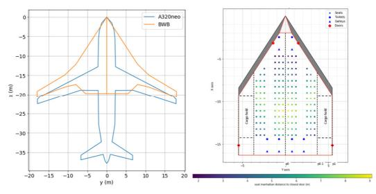
Figure 15 – SMILE configuration top view (left) and pressurized part internal layout (right).
