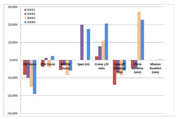
Figure 13 – Comparison of the optimized configurations with the reference configuration.
