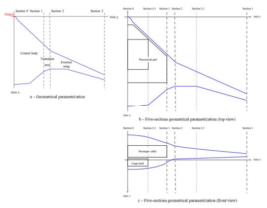
Figure 5 – Geometrical parameterization of the long-range BWB configurations.
