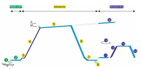
Figure 4 – Mission flight profile modeled with the Mission & Performance Module.
