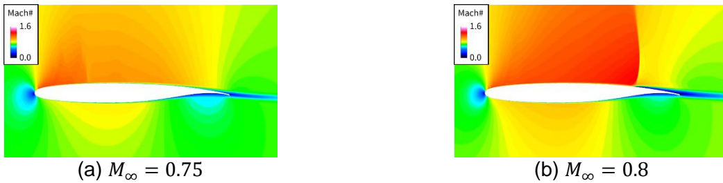
Fig. 4 – Mach number distributions for the SC2-0610 airfoil at the steady-state (non-oscillating) condition around the 1 st -dip.
