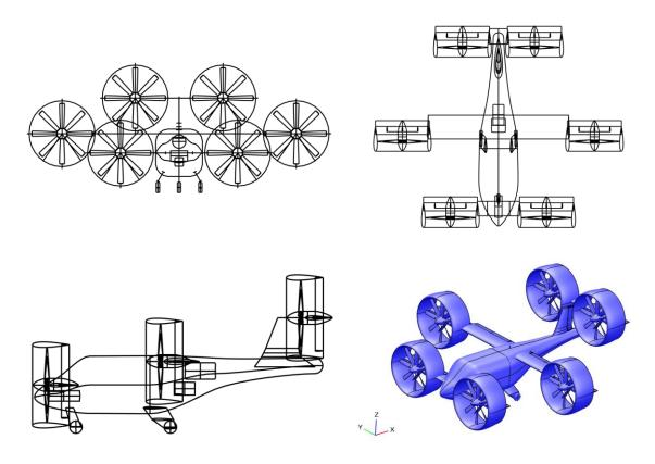
Figure 1 3-D views of NASA UAM tilt-duct eVTOL aircraft, reproduced with NASA OpenVSP, data based on Ref. [11]
