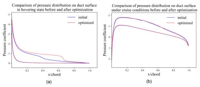
Figure 8 Comparison of pressure distribution on duct surface in hovering and cruise state before and after optimization
