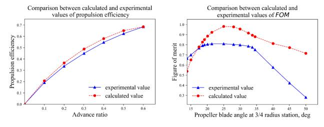
Figure 2 Comparison of DFDC calculated results with wind tunnel experimental results
