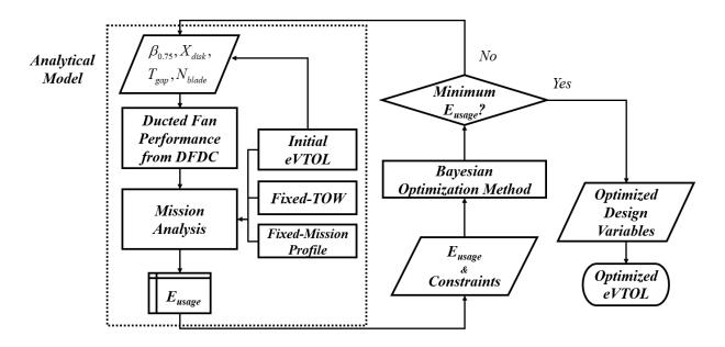
Figure 3 The overall design and optimization process
