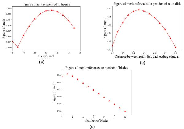
Figure 5 Sensitivity study of FOM depending on tip gap, distance between rotor disk and leading edge, number of blades
