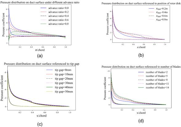
Figure 6 Pressure distribution on duct surface with respect to advance ratio, tip gap, distance between rotor disk and leading edge, number of blades
