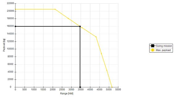
Fig. 3 SAFAM payload-range diagram
