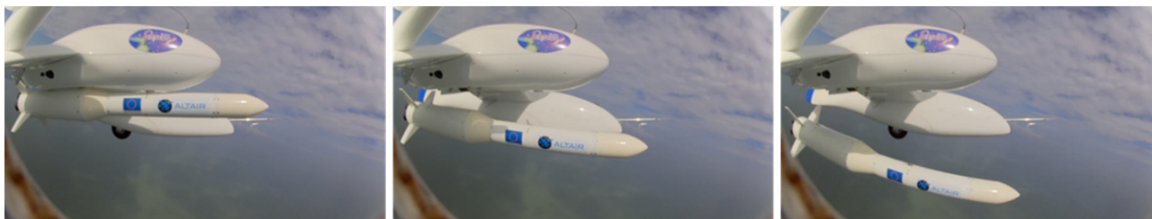
Figure 29 – Pictures of the launcher mock-up separation from the demonstrator EOLE. (credit: ONERA)
