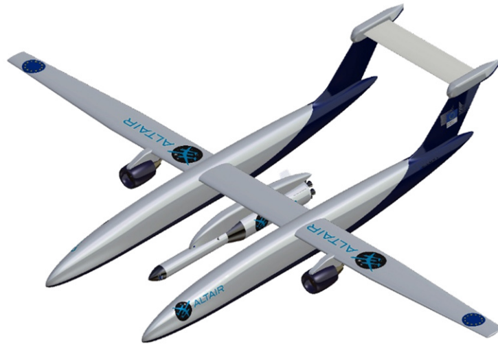
Figure 3 – ALTAIR carrier with the launcher attached under the central pod. (credit: Piaggio Aerospace)
