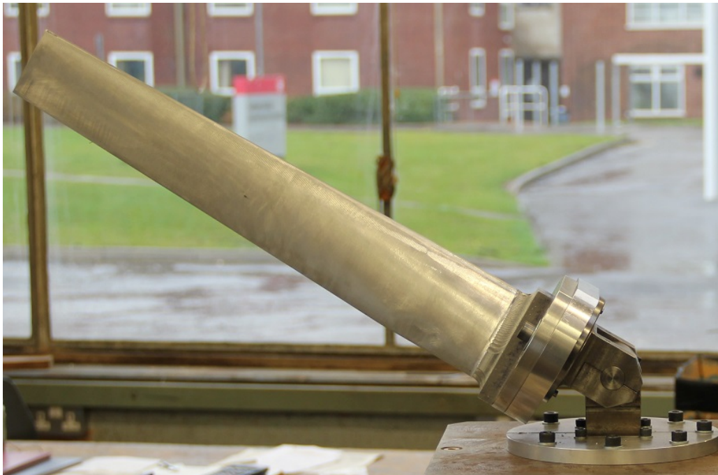
Figure 2 – Image displaying the blade model used in the static blade tests and the pivoting system used to set sweep and incidence angles.
