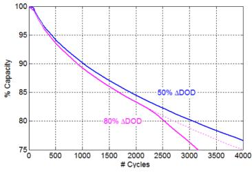
Figure 19. The relation between the number of cycle and charge capacity by effect of depth of discharge.
