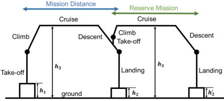
Figure 18. Flight phase of vectored thrust type eVTOL
