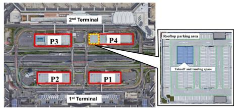
Figure 6. Required area for eVTOL take-off and landing area in rooftop of multi-storey parking building
