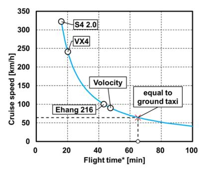
Fig16. Comparison of for different eVTOLs at a specified flight distance.
