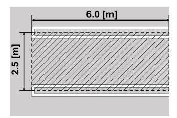
Figure 7. Car parking space dimensions from parking design guideline published by MLIT[6]
