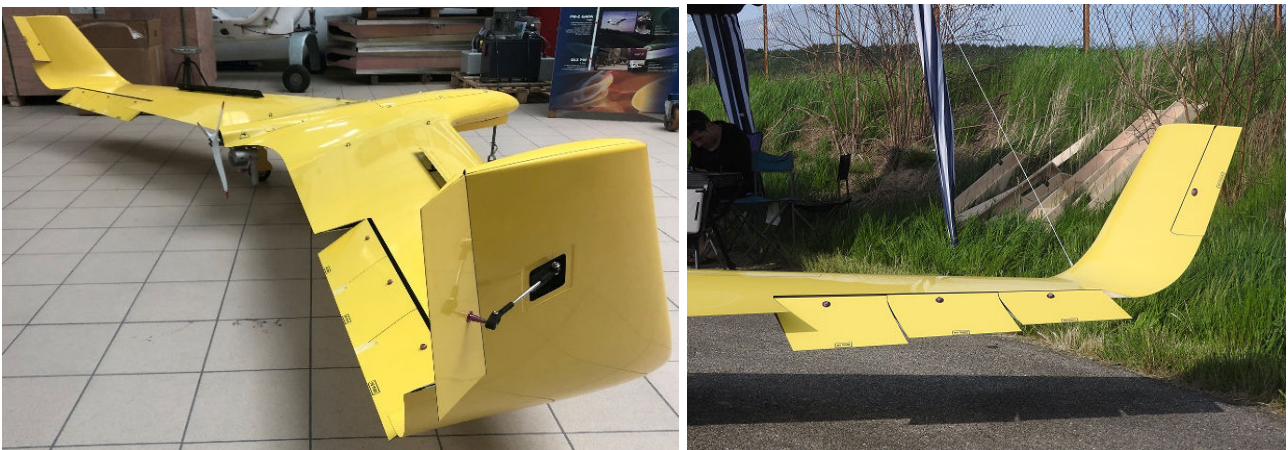
Figure 6 – Control surfaces and winglets tailored for aircraft's optimum performance and stability.
