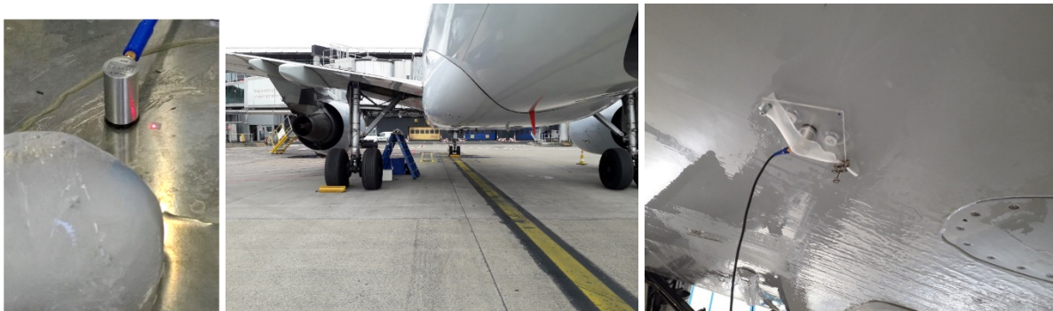
Figure 9 Detection of ultrasonic signals from, resp. “listening” to melting ice at a model tank at lab-scale as well as in future on fuel tanks to determine the moment water draining from fuel tanks can start.
