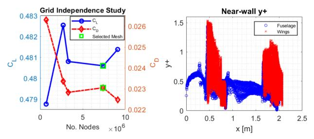
Figure 3 – Grid independence study, final mesh Figure 4 – Near-wall y+ presented alongside the contained 7.6mil nodes.
