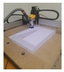
Figure 11 – CNC machine while manufacturing a part of the fuselage.
