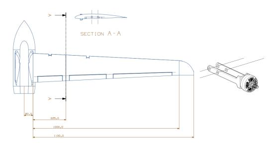
Figure 13 – Drawing of the right wing and fuselage (left) and the motor holder (right). Section A-A is the plane of junction of the wing.
