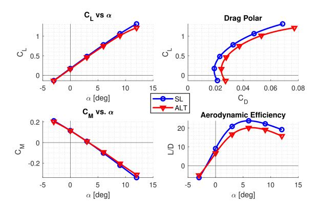
Figure 6 – Simulation results at sea level and at cruise conditions for the final ALPHA design.
