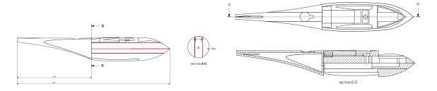
Figure 14 – Fuselage body with (left) and without (right) lids. Red lines indicates manufacturing cutting planes.
