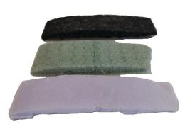
Figure 10 – Wing sample for foam testing - From back to front EPP, PVC and XPS foam.
