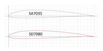
Figure 2 – Aerodynamic efficiency analysis for the final airfoil candidates for ALPHA using XFLR5 (left) and drawing of the SA7035 airfoil (right, top) and SD7080 airfoil (right, bottom).
