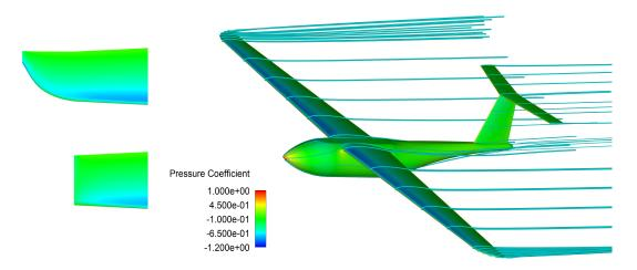
Figure 5 – Pressure contour of ALPHA. Comparison of wing tip versions (left) and streamlines around full configuration (right).
