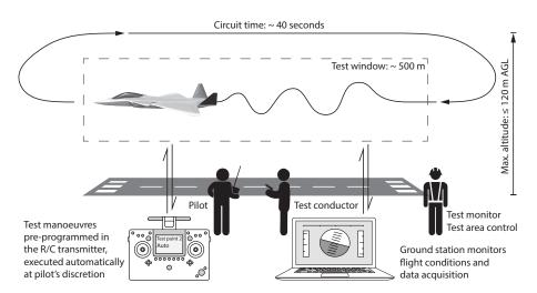
Figure 3 – Cost-efficient flight testing within VLOS using both manual piloting and automation.
