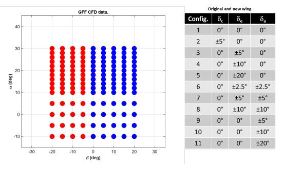
Figure 8 – CFD envelop and control surface configurations.
