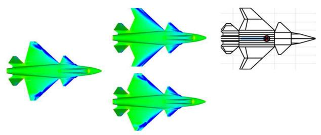
Figure 6 – CFD results used for configuration choice, Euler and panel code.
