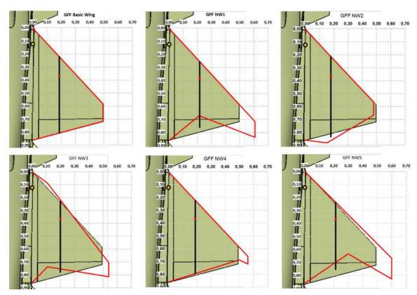
Figure 4 – Wing planform of the original aircraft and the five different concepts.
