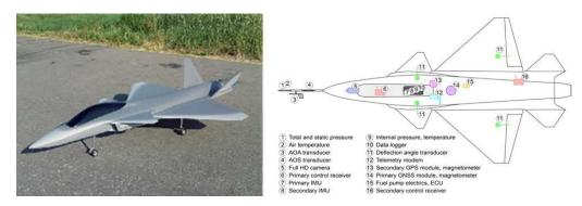
Figure 2 – The GFF aircraft and its data acquisition system.
