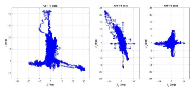
Figure 12 – Flight test envelop and configuration for the original wing configuration.
