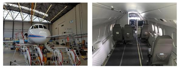
Figure 2 – ISTAR nose boom installation and cabin layout incl. data acquisition system
