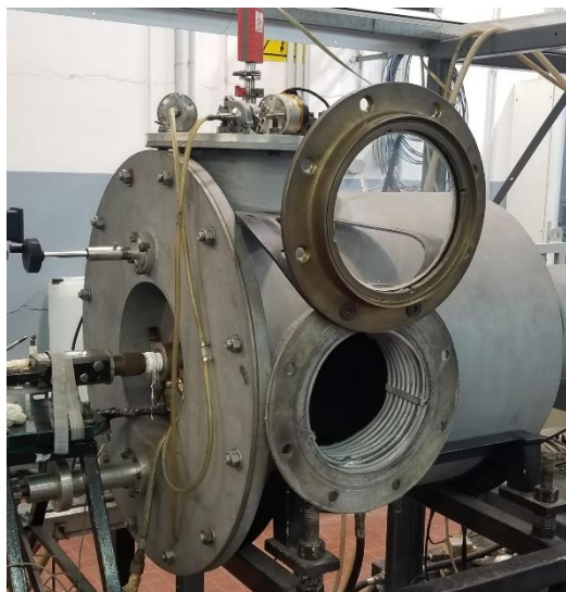
Figure 8 – Vacuum Test Chamber.
