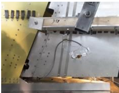
Figure 24 - Strain gauge on the flap skin (left) and hinge moment versus strains, downward and upward rotation together (right).
