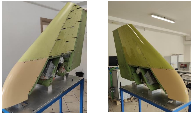
Figure 25 - Final assembly of the left and right IWTs which will be installed on the flying testbed, courtesy of TECNAM
