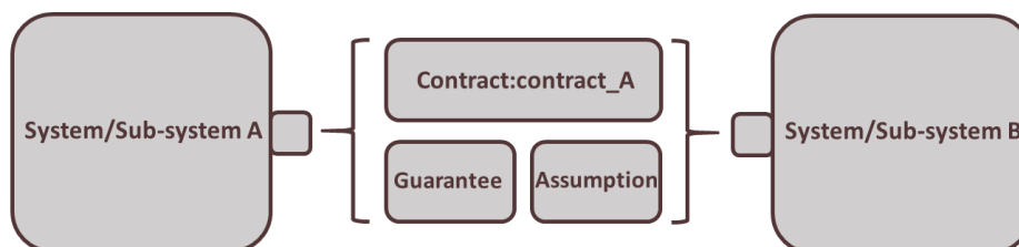
Figure 9. Schematic representation of a contract, including an assumption and a guarantee, between two stakeholders; Stakeholder A is engaged in activities related to System/Subsystem A whereas Stakeholder B is engaged in activities related to System/Subsystem B.
