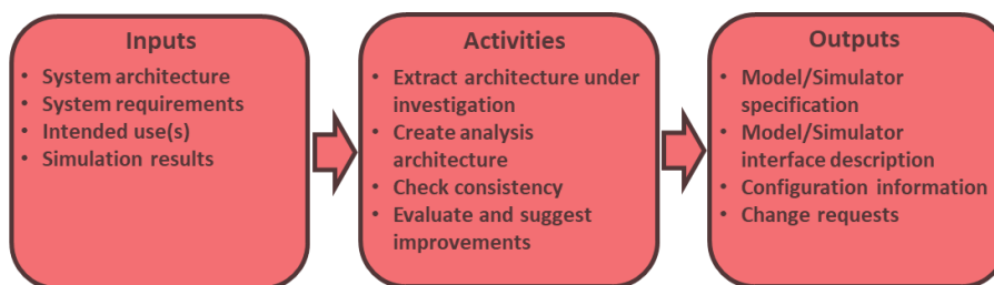
Figure 11. Analysis architecture swimlane as a process in an Input-Process-Output diagram
