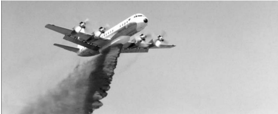
Figure 5 – Water body breakup and diffusion morphology of Lectra L-188 firefighting aircraft.
